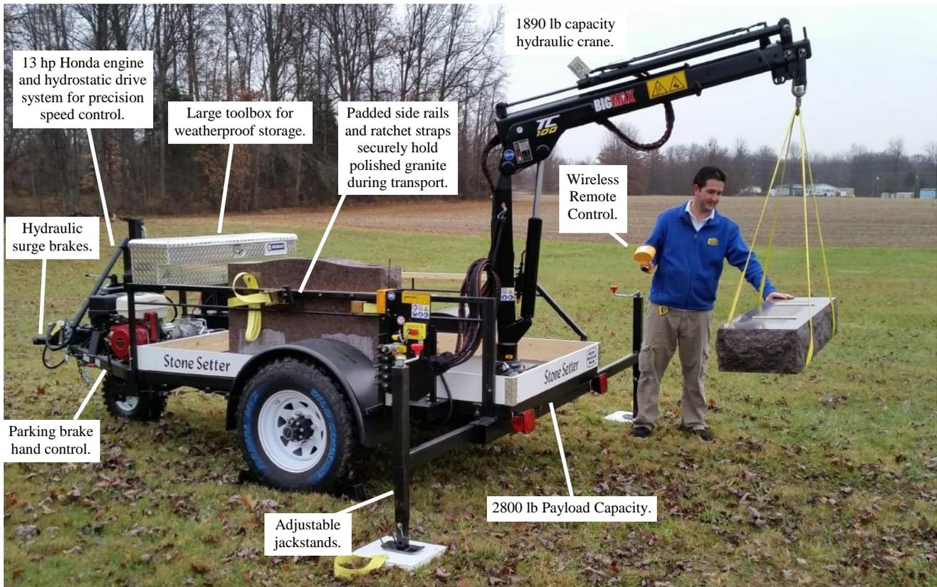
The *Stone Setter* allows one person to do more - quickly, safely, and easily.
