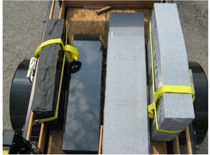
These two double stones weigh 2625 lbs. Max payload is 2800 lbs.
